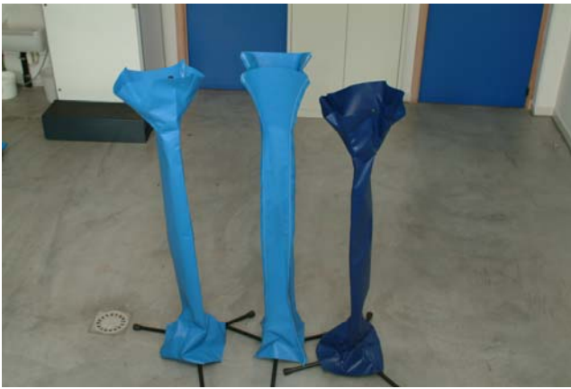
Figure 8: Prefabricated fabric moulds for columns.
