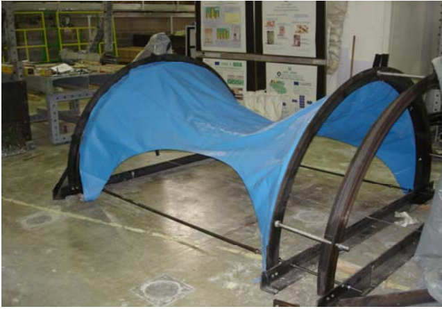
Figure 13: Fabric formwork, pretensioned using a secondary structure.
