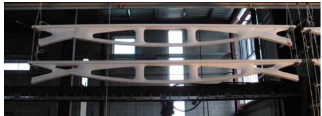
Figure 2: Plaster models of lightweight trusses made with fabric formwork (West 2006).
