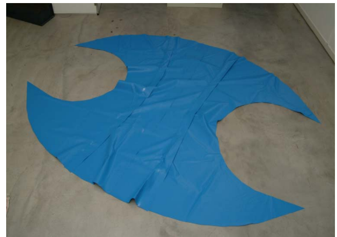
Figure 12: Fabric formwork for the double-curved shell.
