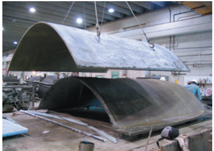
4. A thin-shell GFRC vault is produced from the fabric-formed mold.
