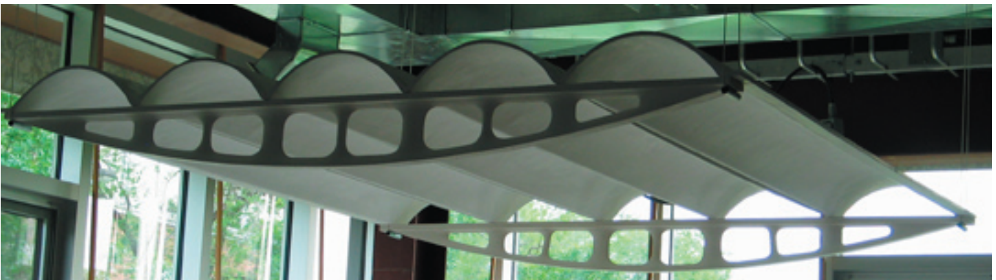
5. Plaster model of a precast funicular vault structure (supported here by fabric-formed prestressed plaster trusses). C.A.S.T. Laboratory 2007
