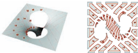
Figure 9: Cutting pattern of 18 panel shapes (x2).
