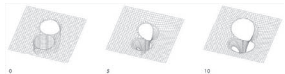
Figure 4: Number of form-finding steps in development of minimal surface.
