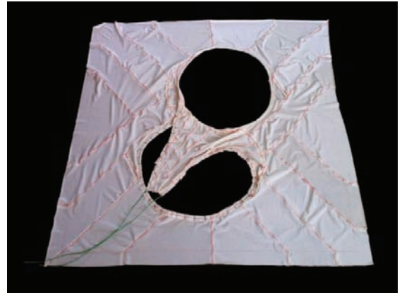
Figure 10: Membrane of sewn panels ready for mounting on tension frame.
