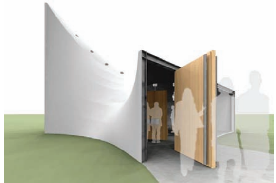
Figure 17: Exterior rendering of chapel using mechanical tensioning defining a minimal surface.
