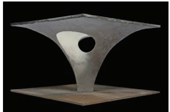
Figure 15: Finished mock-up in poured gypsum.
