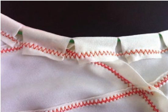
Figure 8: Cable pocket sewn into fabric edge.
