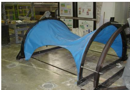
Fig. 8: Pretensioning the fabric with a secondary structure.
