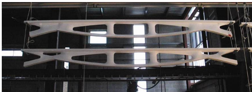
Fig. 1: Plaster models of lightweight trusses made with fabric formwork (West 2006).
