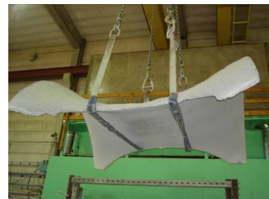
Fig. 10: Shell after demoulding.
