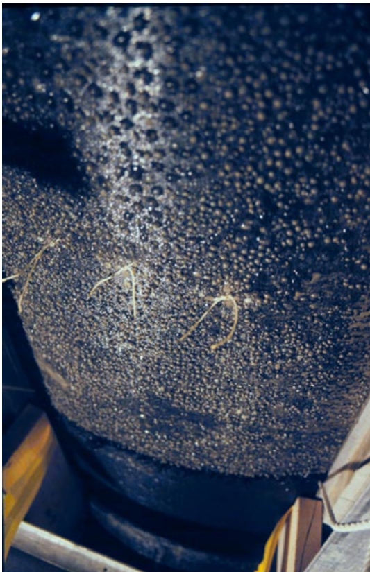
Figure 11. Filtration of excess water and air bubbles through geotextile fabric (C.A.S.T. photo).
