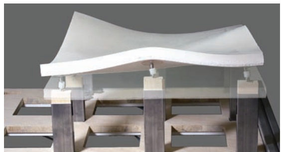
Figure 9: Step 2, adjustable mold actuation.
