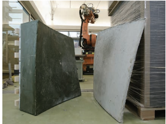
Figure 7: Prototype for testing of the wax material properties. Wax formwork (left), concrete cast positive (right).
