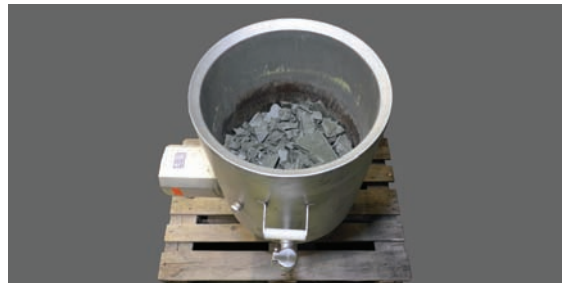
Figure 8: Step 1, melting re-used wax.
