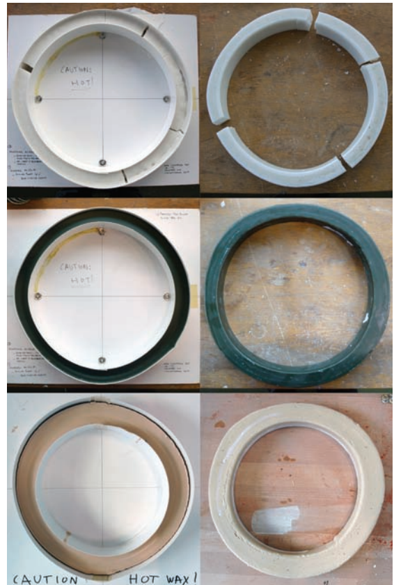
Figure 4: Ring shrinkage tests of different wax types. From top to bottom: High melting point polymer wax with shrinkage cracks, investment casting wax without shrinkage cracks, custom formulated concrete casting wax without shrinkage cracks.
