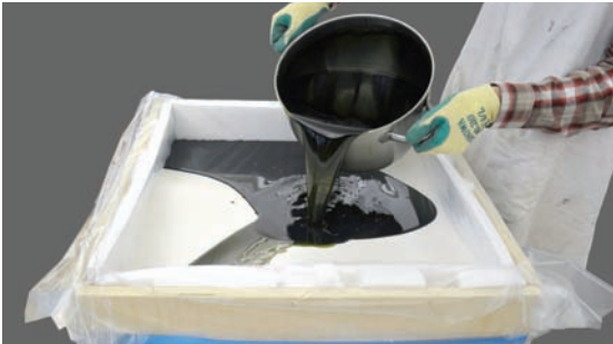
Figure 10: Step 3, casting hot wax in mold.
