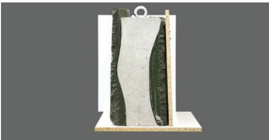
Figure 12: Step 5, wax formwork on-site.
